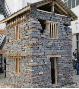
Test Set up and Wall tested on Stone in Mud with Wooden Bands
